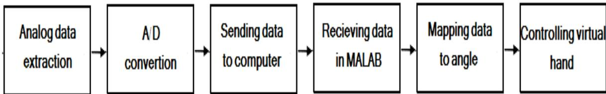
Fig. 13. All needed steps to simulation
