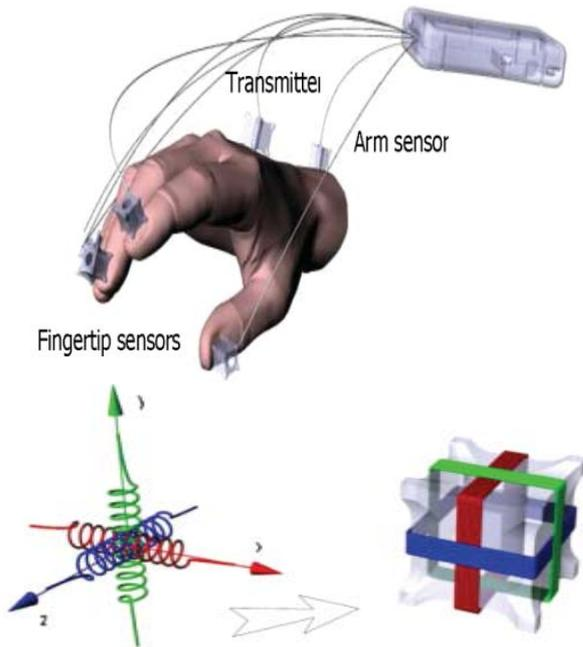
**Fig. 3.** Coils placement on the hand and Orthogonal coils antenna for transmitter/receiver [4].
