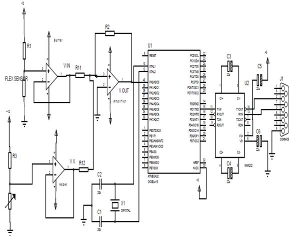
**Fig.9.**Circuit of the extraction [14], digitization, sending and conversion to computer-usable data for one sensor
