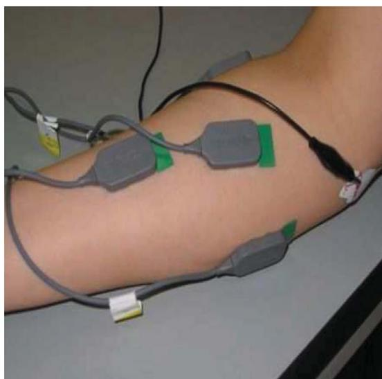
Fig. 6(a). Surface EMG sensors
