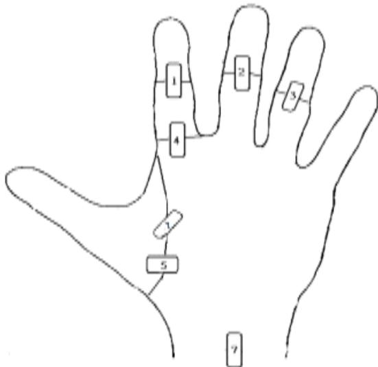
**Fig.8.** Positions of the sensors on the data glove [1].
